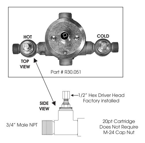
Note: The Standard 7-1/4"Cover Plate does not provide proper access to these shut offs.
